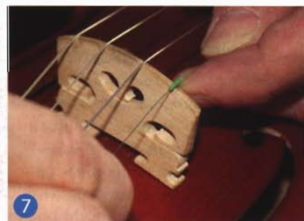
7 Place the damper: Steel strings, like this high E, often have a damper; this goes into the slot where the string meets the bridge.
