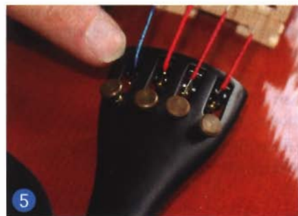
5 Mount the ball end on the bridge: Before the string is completely tight, slot it into the tailpiece.
